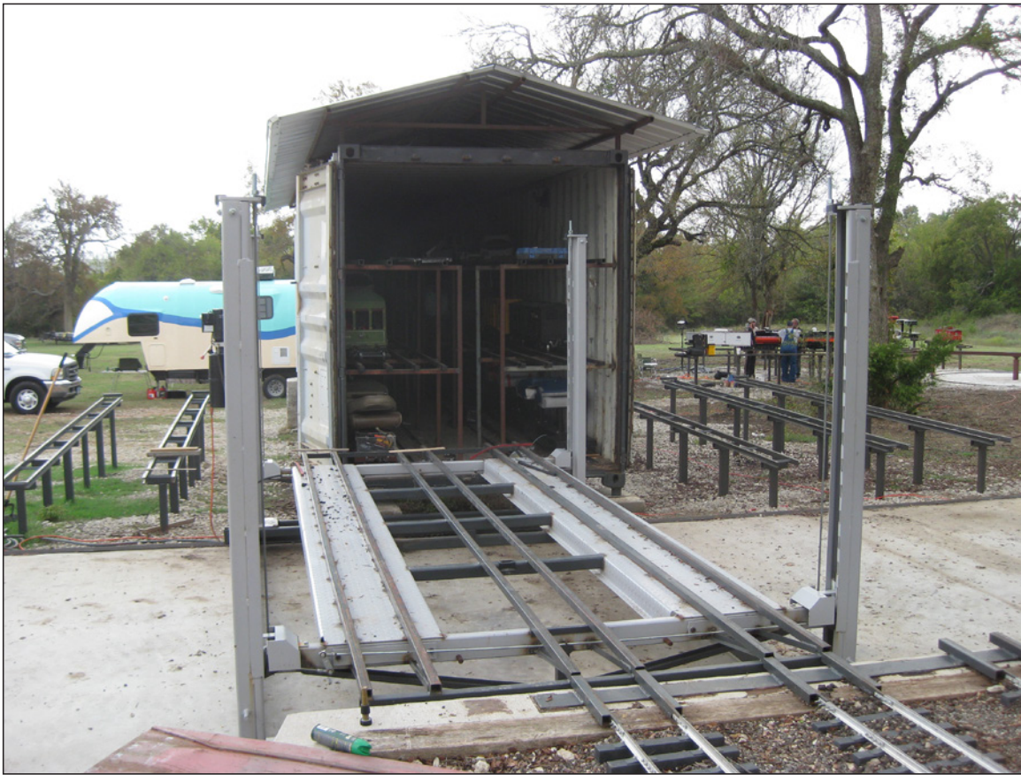
Figure 2: Three-track transfer table
